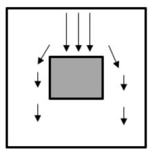
Plan view of BESS foundation below ground showing the water flow pathways
